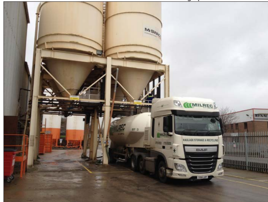
Milled barite loading operations at Aberdeen
