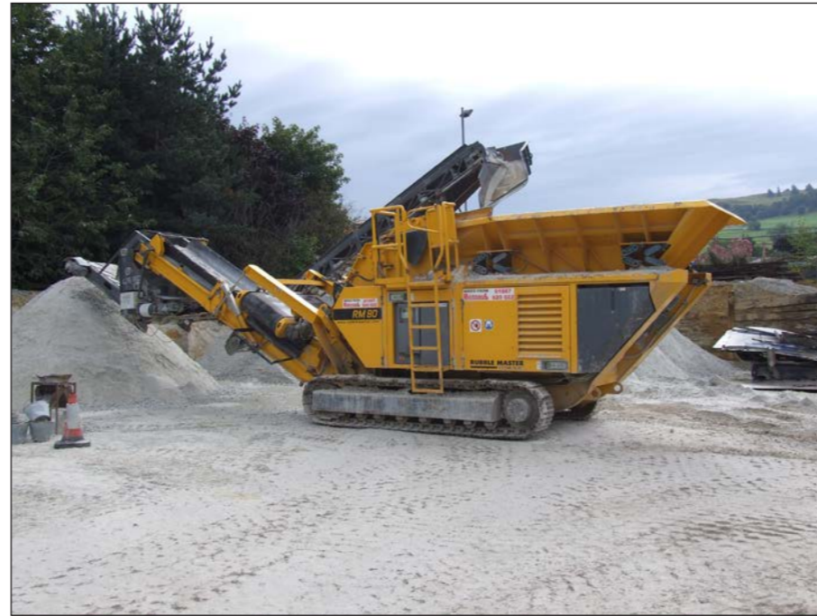
Barite crushing at the Aberfeldy yard
